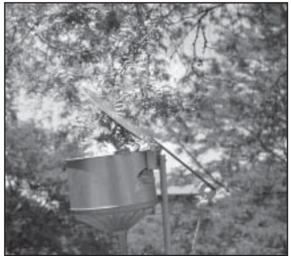
Figure 1. Modified funnel on extension pole used to sample insects in honeylocust trees.
