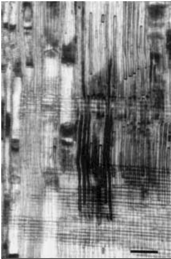
Figure 2. Radial longitudinal section through a reaction zone in sycamore ( Acer pseudoplatanus ), showing colored polymeric deposits occluding the lumens of vessels and xylem fibers, and infiltrating the wood cell walls in this region. Scale bar = 100 \mu\text{m} .
