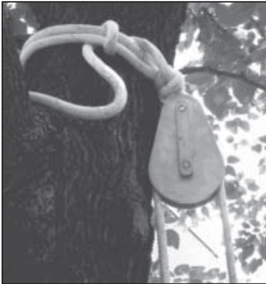
Figure 1. Photograph of an arborist block installed in a tree. A 19-mm (3/4-in.) double-braid polyester sling with an eye spliced in one end is affixed to the block and tied with a cow hitch to the main stem. A second 14.3-mm (9/16-in.) double-braid lowering line is run from the back (left in this figure) and over the sheave. The working end of the lowering line is to the right, and the running end is to the left. Note how the cheek plates of the block will protect the line from abrasion with the trunk.
